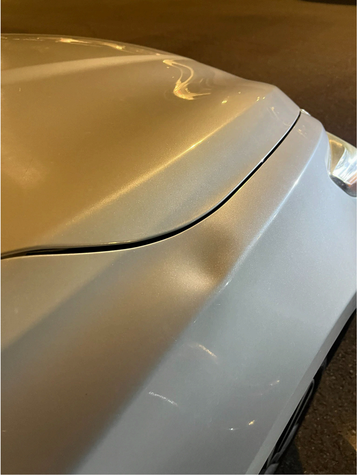
Damage to vehicle reportedly caused by baseball impact during practice activity.
